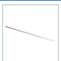
Pipe of 42 mm diameter with rotary clamp used for scaffolding stiffening. To be assembled by fitting the top brace end into stiffening sheet of vertical frame and fastening the opposite end with clamp at the bottom of the opposite vertical frame.
