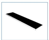
Aluminium-plywood platform with waterresistant plywood of rough surface. Finished with three holders on each side for hanging on the frame U-profile, thus assuring optimal safety level for the user. Platform width corresponds with complete working platforms for 0.73 m wide frames. Aluminium platform of 0.61 m width supersedes two steel platforms 0.32 m wide maintaining allowable load upto 2 kN/sqm and lowering total weight of platforms by 50 per cent.
