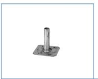
Foot sized 150 x 150 mm with pipe stem of 36 mm diameter used for correct positioning of the scaffolding which requires no levelling.
