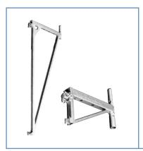
Fastened to vertical frame at the level of stiffening sheet with rotary clamp which is fixed to the bracket. Allows for widening of scaffolding by 0.36 m, 0.73 m or 1.09 m. Permissible bracket load:
