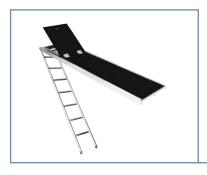
Underslung platform ladders ensure easy horizontal traffic along scaffolding levels. Load-bearing structure and integrated ladder made of aluminium. Filled with water-resistant plywood of antislip surface. Used for in-scaffolding
