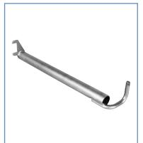
Pipe of 48 mm diameter provided with hook and sheet to be fit under the frame U-profile. It is fixed in the stiffening sheet cuttings with one normal coupling and regulates the distance between the wall and the scaffolding carrying the external load from the scaffolding onto the building.
