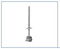
With threaded pipe plunger, nut and clamp on pipe of 48.3 mm diameter. Tilt mounted on foot of 150 x 150 mm. Used for frame positioning on sloped surfaces.
