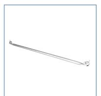
Pipe of 48.3 mm diameter with normal semi-coupling (nut and bolt) permanently fixed at the ends of brace. Mounted with semi-couplings to the opposite vertical frames. Serves as the stiffener of scaffolding structure.
