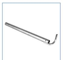
Long anchor coupling links 1.30 m and 1.50 m long fastened with two normal couplings to both stands of vertical frames. Short anchor coupling link 0.40 m long fastened with normal coupling to one frame stand next to the wall.
