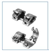
Used for coaxial, in-line connection of two pipes of 48 mm diameter. The in-line coupling must be made with aligning pin fixed in the contact point of two pipes. Permissible load of in-line coupling equals to 6 kN.
